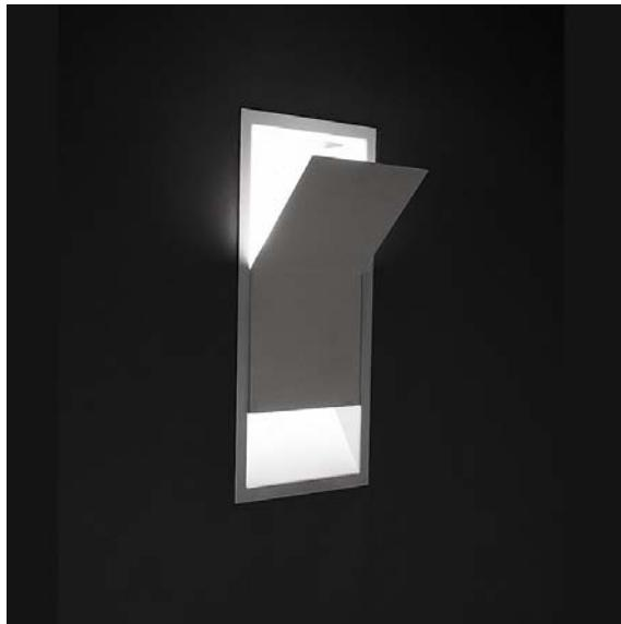
indoor recessed light fixture IP20 with double emission made of white or grey painted metal. it can be used in brick walls, thanks to the special housing, and in plasterboard. it takes R7s-114 150W linear halogen lamps.
