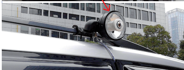
A sensor module mounted to the roof of a car captures the optical condition of a gas pipeline in China as the car passes by.
