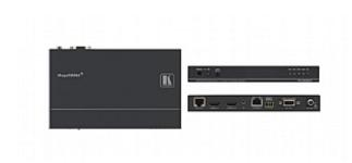
The TP-582T is a high-quality twisted pair transmitter for HDMI, Ethernet 100BaseT, bidirectional RS-232 and IR signals. The TP-582T selects one of two HDMI inputs, and converts it with the Ethernet 100BaseT, RS-232 and IR input signals to an HDBaseT twisted pair signal. The TP-582R converts the HDBaseT twisted pair signal back to Ethernet 100BaseT, RS-232, IR and two HDMI outputs, and de-embeds the audio to S/PDIF and TOSLINK® audio outputs.
