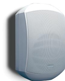
The MASK6 is a 6.5" two-way low impedance loudspeaker with timeless design. This full range loudspeaker has been designed for the contractor market and delivers crystal clear sound, from background music up to 'dance level' music. It can of course be used with a subwoofer when higher power is needed. MASK6 loudspeakers are suitable for both indoor and outdoor use (IP64 rating).
